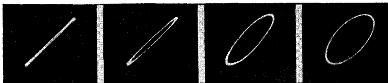
Figs. 217, 218, 219, 220, reading from left to right. Oscillograms showing varying degrees of loss and power factor in condensers. The greater the area of the ellipse, the higher the losses and the higher the power factor.
