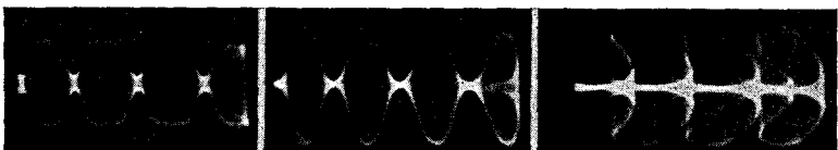
Figs. 433 (left), 434 (middle), 435 (right). When the audio leads, which were the cause of the distorted pattern of Fig. 432, were removed, the pattern of Fig. 433 was obtained, this being the correct one. Before the audio leads were removed in a similar case, the pattern of Fig. 435 was on the screen, the corrected pattern being shown in Fig. 434.
