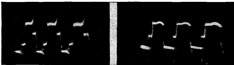
Figs. 378, left, 379, right. The waveform taken in the primary circuit when the buffer condenser was removed is shown in Fig. 378. The waveform of the secondary circuit under similar conditions is shown in Fig. 379.
