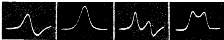
Figs. 286-A, 286-B, 287-A, 287-B, from left to right. The oscillograms of Figs. 286-A and 287-A show phase distortion in single peaked and double peaked curves, respectively. Correct corresponding curves with no phase distortion are shown in Figs. 286-B and 287-B.
