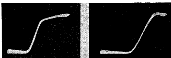
Fig. 132, left, Fig. 133, right. Tube characteristics obtained when the filament, grid and plate voltages were held constant and changes made in the load resistance, R_1 of Fig. 128. The pattern of Fig. 132 was photographed when R_1 = 0 and that of Fig. 133 when R_1 = 10,000 ohms.
