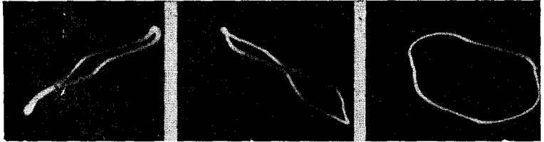
Fig. 95. E, left, F, middle, G, right. The three Lissajous figures here shown indicate a 1-1 ratio. One of the voltages impressed on the plates was not a pure sine wave; hence the distortion.
