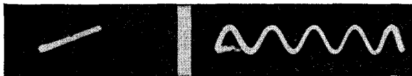
Figs. 181, left, 182, right. The input-output voltage characteristic for distortionless operation is shown in Fig. 181. That it is distortionless is shown by the undistorted sine wave output of Fig. 182.
