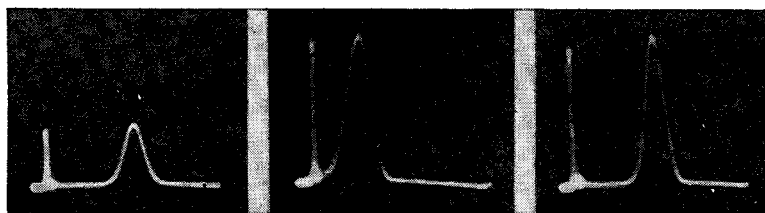
Figs. 445, left, 446, middle, 447, right. Fig. 445 shows an incorrect adjustment of the padding condenser, whereas Fig. 446 shows the correct adjustment. In Fig. 447 the tuning has been changed to bring the peak to the center of the trace.
