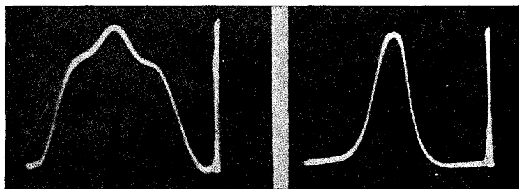
Fig. 276, left, Fig. 277 right. The resonance curve in Fig. 276 is non-symmetrical and that in Fig. 277 is symmetrical. These oscillograms were made using the frequency modulator and sweep described in Fig. 275. The vertical line on the right of each oscillogram indicates the vertical displacement due to change in frequency, but as the sweep was shortened, it is not spread across the screen.
