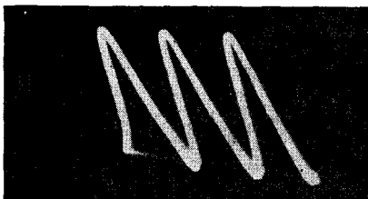
Fig. 138, left. When the sweep frequency was increased after the pattern of Fig. 137 was photographed, the three cycles of the wave, shown on the left, indicate the necessity for having the deflecting coils properly oriented with respect to the sweep
