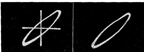
Fig. 93-G, left, Fig. 93-H, right. Pattern for a phase difference of approximately 135°. The pattern of H is the same as that of G with- out the horizontal and vertical refer- ence axes.
