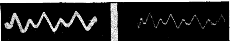
Figs. 372, left, 373, right. Oscillogram of voltage taken across V and V1 is shown in Fig. 372. Fig. 373 shows the voltage across the same points, but with a shorter exposure of the photographic film. Note the transients in Fig. 372, indicated by the faint vertical lines below the wave, but not visible in Fig. 373.
