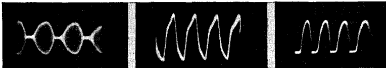
Fig. 232-A, left, Fig. 232-B, middle, Fig. 232-C, right. A. The wave envelope of the modulated output of a commercial test oscillator. B. The a-f. output of the same oscillator. C. The a-f. signal resulting from demodulation of the modulated wave shown in A.
