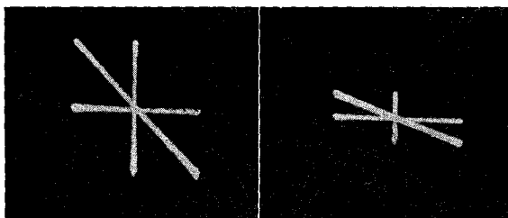
Fig. 93-C, left, Fig. 93-D, right. A phase difference of 0^\circ exists between the two voltages. In C equal amplitudes on both axes give the pattern a 45^\circ angle with the horizontal, but when the horizontal amplitude is increased, as in D, then the pattern approaches the X-axis.
