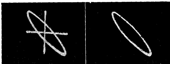
Fig. 93-E, left, Fig. 93-F, right. Pattern for a phase difference of about 45^\circ . Both E and F are the same pattern, but the X and Y axes were omitted from F.
