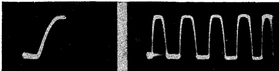
Figs. 185, left, 186, right. A further increase of input to the amplifier developed the characteristic of Fig. 185. That the positive swing was excessive was proved by the output waveform of Fig. 186.
