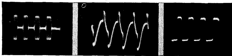
Fig. 230-A, left, Fig. 230-B, middle, Fig. 230-C, right. A. The wave envelope of the modulated output of a commercial test oscillator. B. The a-f. output of the same oscillator. C. The a-f. signal resulting from demodulation of the modulated wave shown in A.
